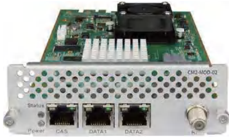
CM2-QAMA-02/02A CM2-QAMB-02/02A IPQAM Module
