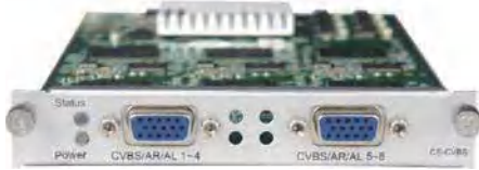
CE2-CVBS-R01: Commercial CVBS Encoder Module
