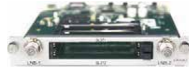
CR2-DVBS2CI-01: DVB-S/S2/S2X with CI Receiver Module
